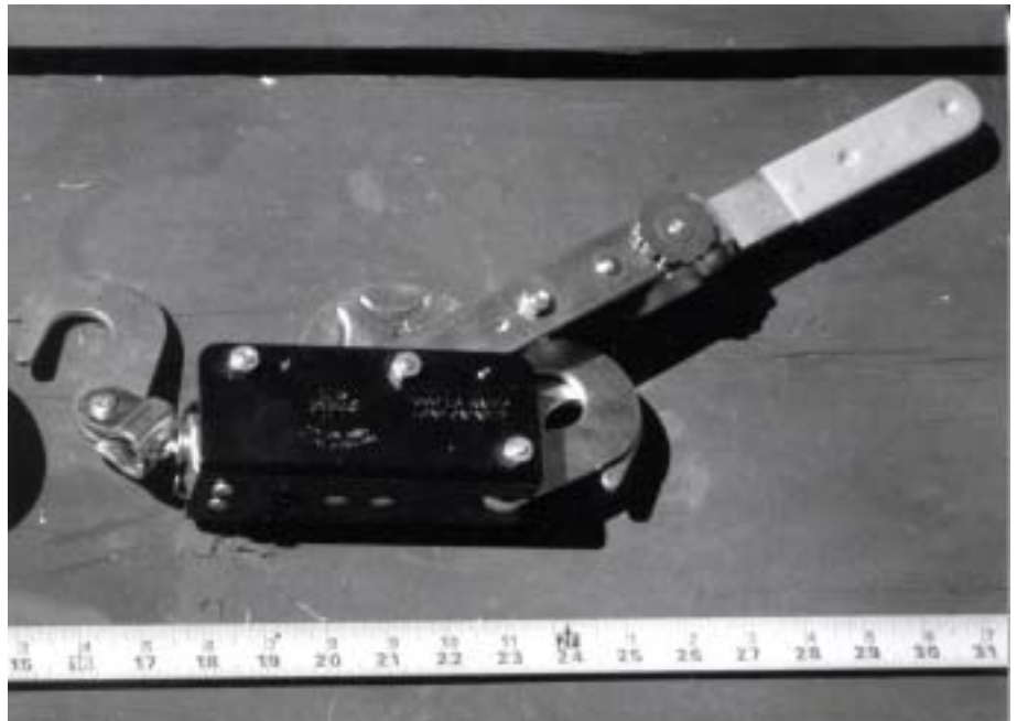
Figure 6.—Portable hoist/puller did not work well in field tests.
