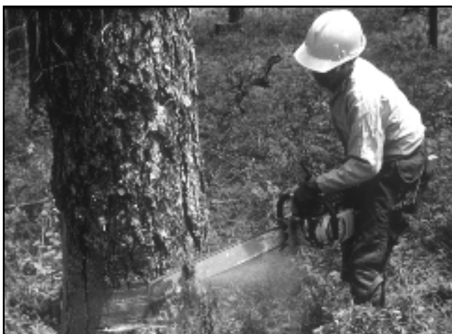
Figure 3-22—Bark can be removed with the tip of the bar.
