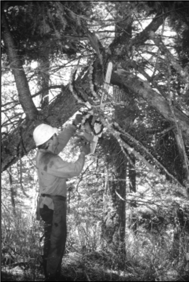
Figure 3-9—Do not cut with the chain saw above shoulder height. Keep the chain saw below your shoulders to maintain control when cutting.
