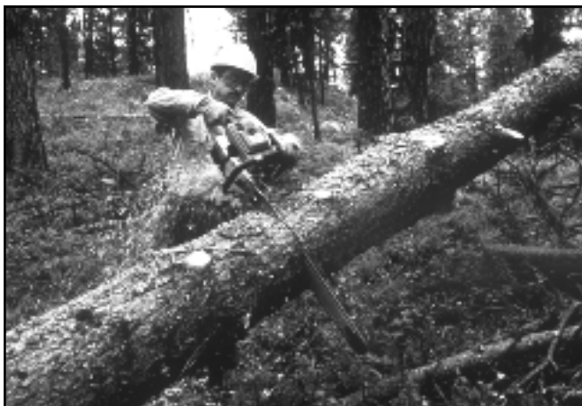
Figure 3-8—The top side of suspended logs should be limbed on the top side while you are standing on the ground or lower the log to the ground by bucking.
