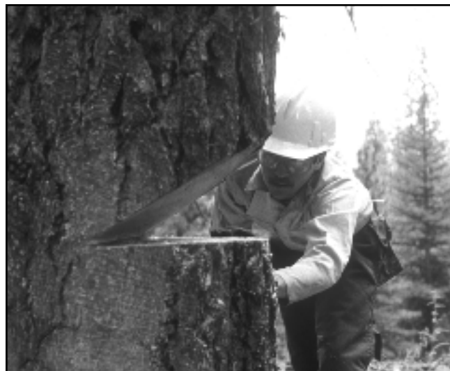
Figure 3-23—The sloping cut is a 45-degree angle.
