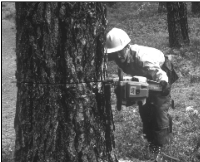
Figure 3-25—Use the gunning marks to check the felling direction.
