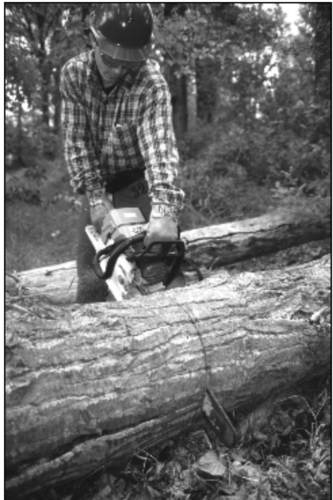
Figure 3-5—Watch the kerf for movement that will indicate a bottom bind (kerf opens) or top bind (kerf closes).
