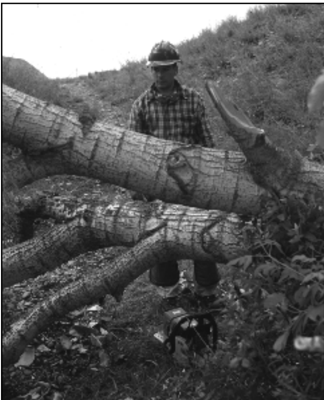
Figure 3-4—Determine and stay clear of the offside (downhill side) when you are bucking.
