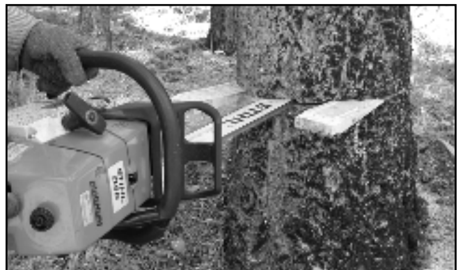
Figure 3-19—Complete the backcut.
